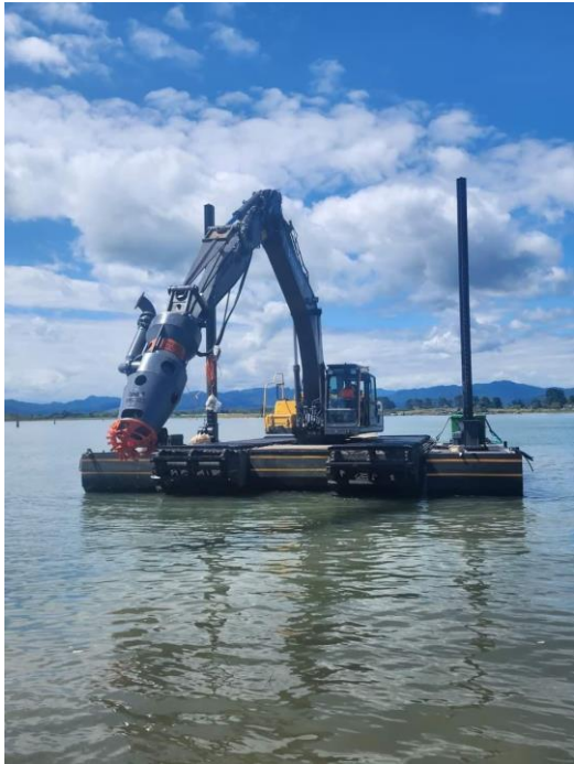
Image shows amphibious configuration with additional sides, centre pontoons and rear 10m hydraulic spud
